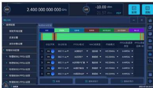
WLAN physical frame block configuration interface
