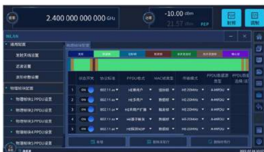
WLAN physical frame block configuration interface
