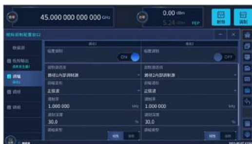
Analog modulation configuration interface
