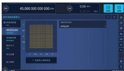
4096QAM modulation configuration interface
