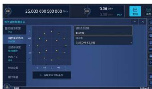
16APSK modulation configuration interface
