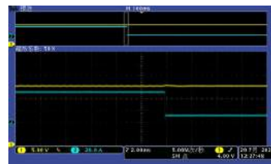
50% to 10% load change: Dynamic response waveform
