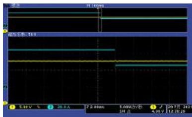
90% to 50% load change: Dynamic response waveform
